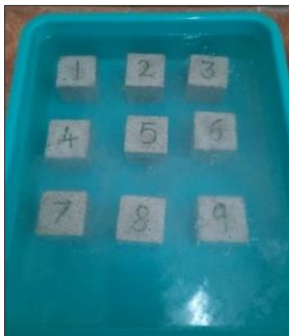
Figure 10. 40mm cubes immersed in water
