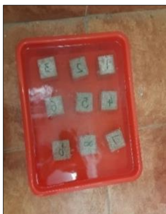
Figure 11. 40mm cubes immersed in 5% dil. Nitric acid
