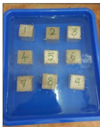
Figure 12. 40mm cubes immersed in 5% dil. Sulphuric acid
