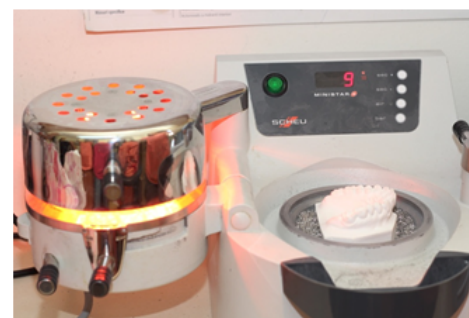
Fig. 2. The manufacturing of the trays: the Ministar vacuum-forming device
