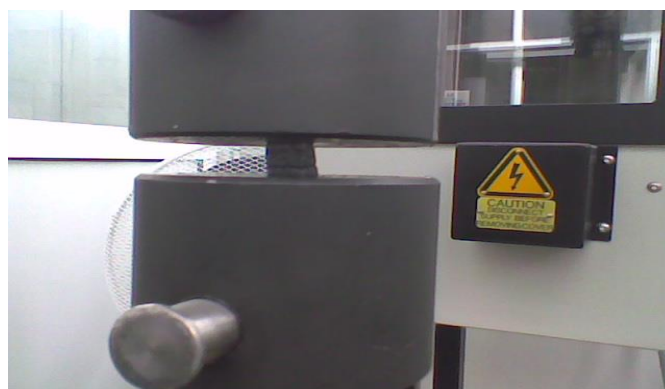
Figure 1. Testing machine with the specimen mounted between the compression jaws of the test device
