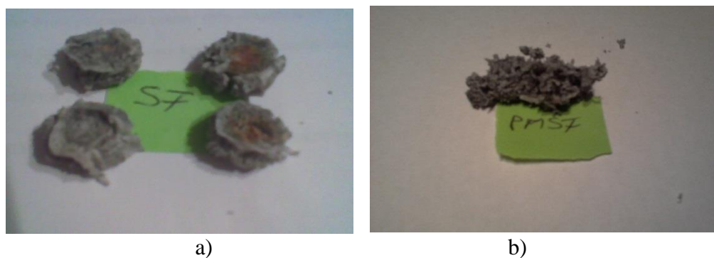
Figure 6 The appearance of specimens after compression testing a) composite material without metallized mesh; b) composite material with metallic mesh
