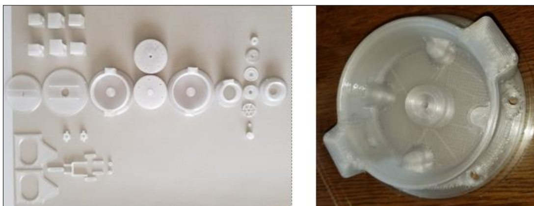
Figure 16. Almost all the 3D printed components of the fertigation pump
