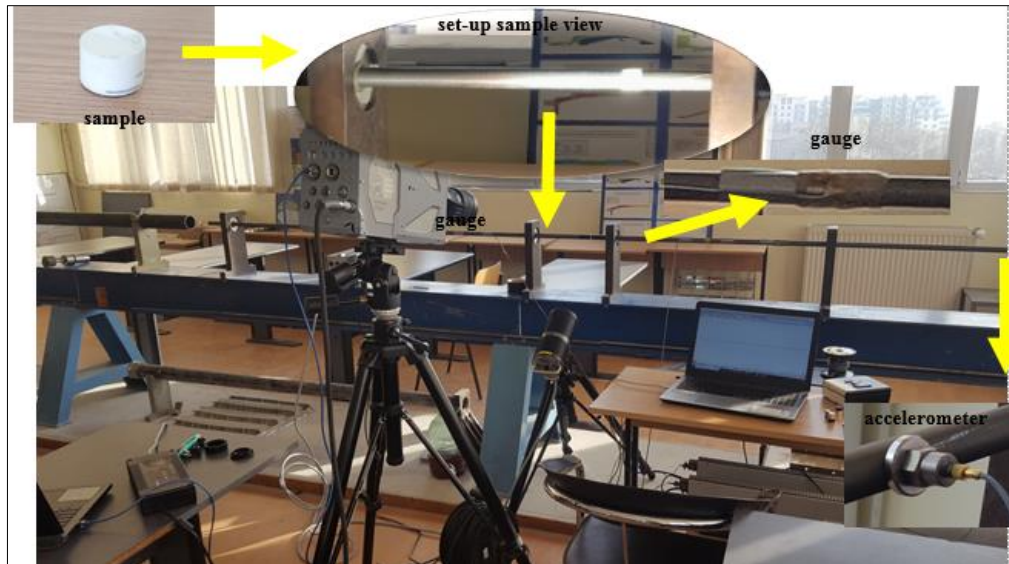
Figure 3. Experimental set-up for compression tests with Split Hopkinson pressure bar
