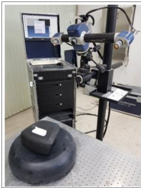
Figure 9. 3D scanning for checking dimensional accuracy
