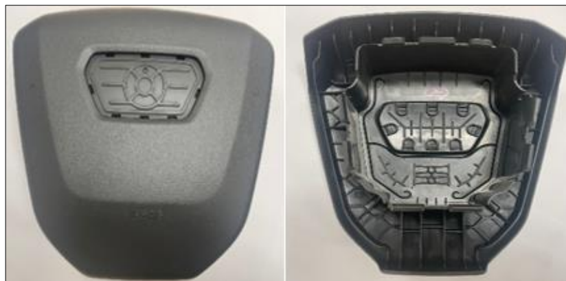
Figure 15. Final molded horn cover: (a) front (b) back
