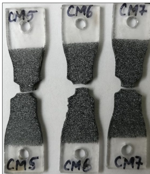
Figure 9. Tested samples with stress concentrators
