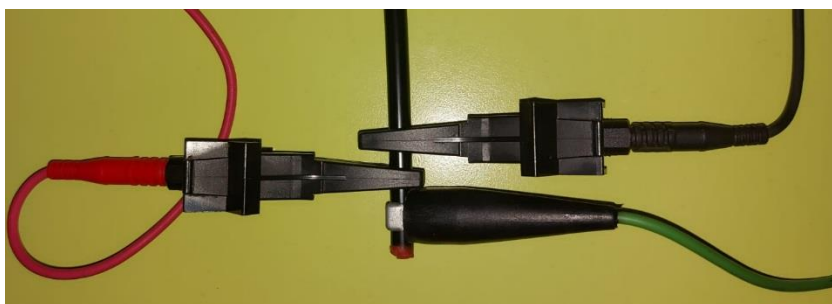
Figure 1. Electrodes placement during the electric resistance measurements
