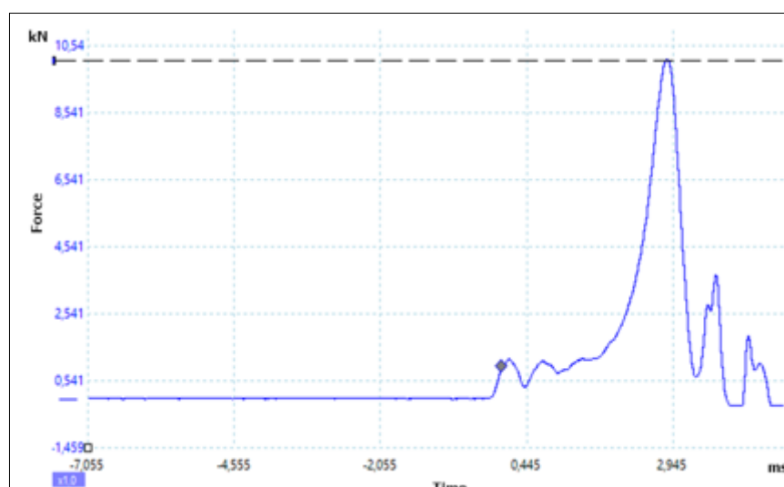
Figure 4. Typical example of force vs time signal
