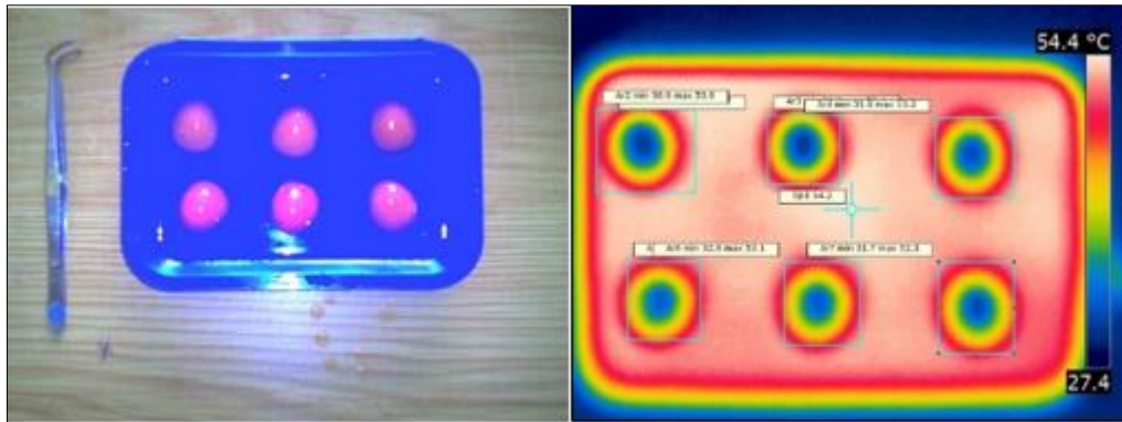
Figure 3. The saline solution tray with the partially immersed 6 replacement prostheses in normal and infrared image
