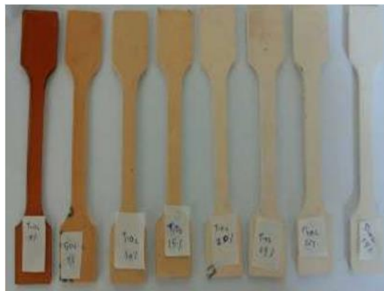
Figure 7. Tensile test samples (PU+(0-35% TiO 2 ))
