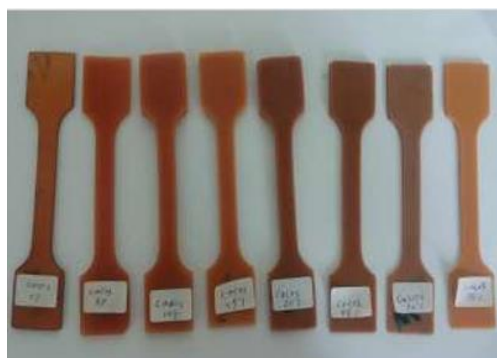
Figure 6. Tensile test samples (PU+(0-35% CaCO 3 ))
