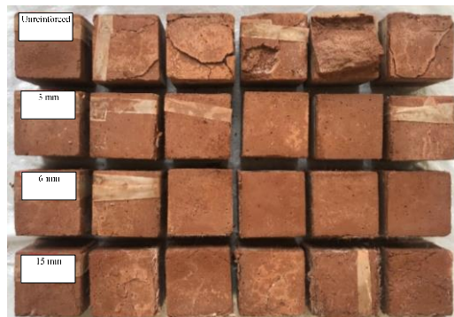
Figure 5. Photograph of specimens after 21 cycles of freezing and thawing
