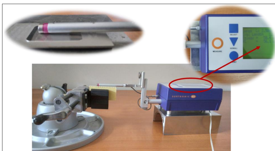
Figure 5. Surface roughness measurement procedure
