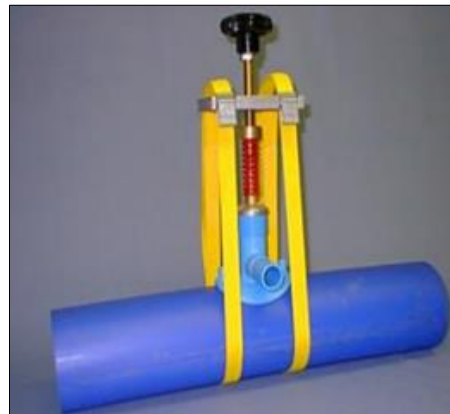
Figure 4. Device for fixing a saddle tee [12]
