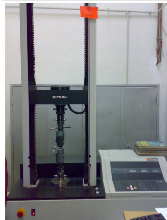
Figure 26a. Machine for testing tensile, compression and Buckling strength Instron 4303
