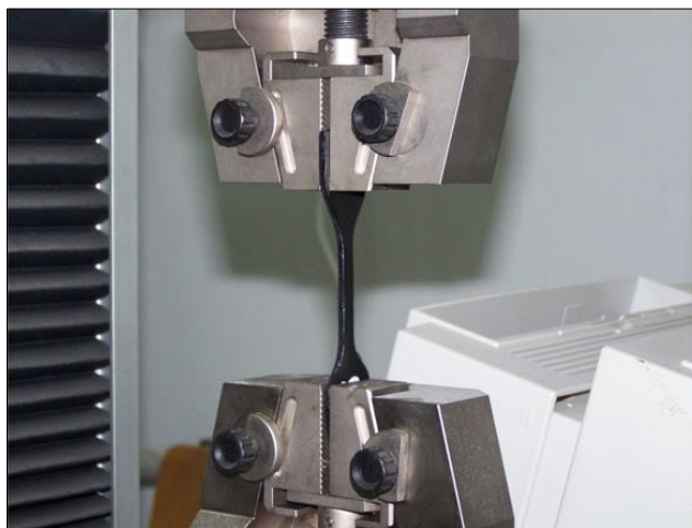
Figure 28. Fastening the pipe in the grips of the testing machine
