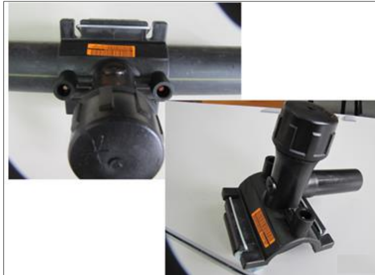
Figure 3. Polyethylene fitting 63-32 mm in diameter, before and after welding
