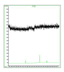
**Figure 1.** 3 ppm standard solution chromatogram overlay (green)/ solvent chromatogram (black)
