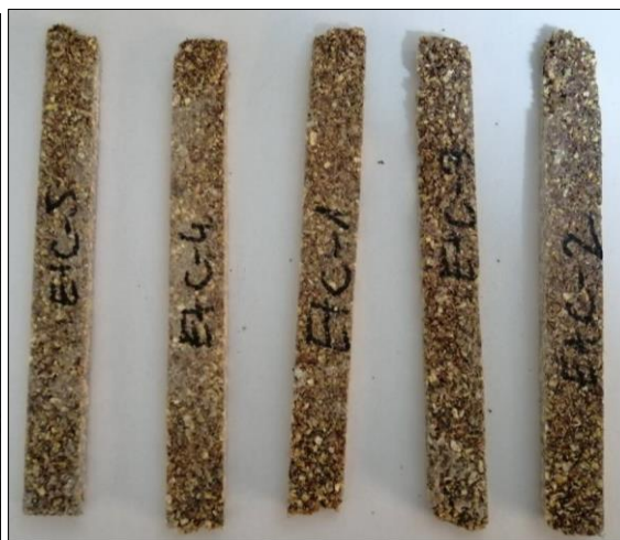
Figure 2. Some samples used for the tensile test
