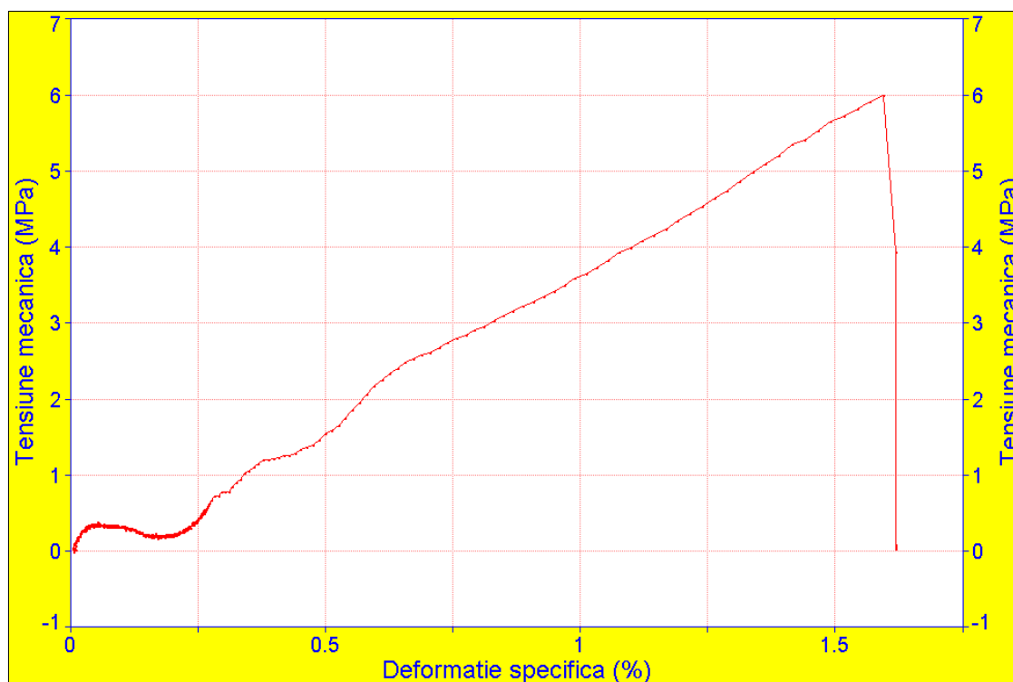
Figure 4. The Hooke graphic for a representative sample, tensile tested
