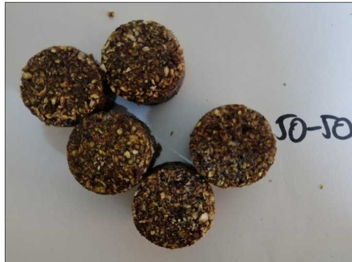
Figure 3. Some samples used for the compression test, with 50% corn cob powder
