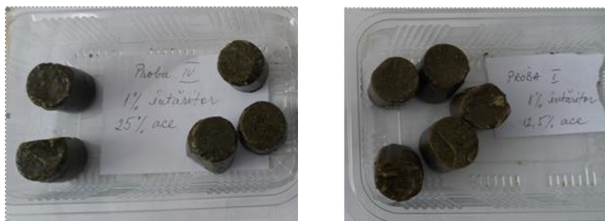
Fig. 3. Two types of version A specimens with the next fir needles powder content percentages: a) 25%, respectively b) 12.5%
