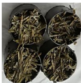
Fig. 4. Version A specimens with different whole fir needles content percentages
