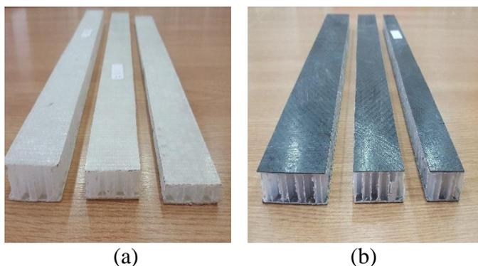
**Figure 3.** Medium-layer polypropylene honeycomb bars and outer layers with fiberglass (a) and carbon fiber fabric (b)
