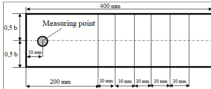
**Figure 4.** Position of the measuring point where the accelerometer was located
