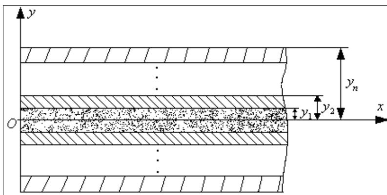
**Figure 1.** Sandwich bar with geometric and massive symmetry to the middle layer.
