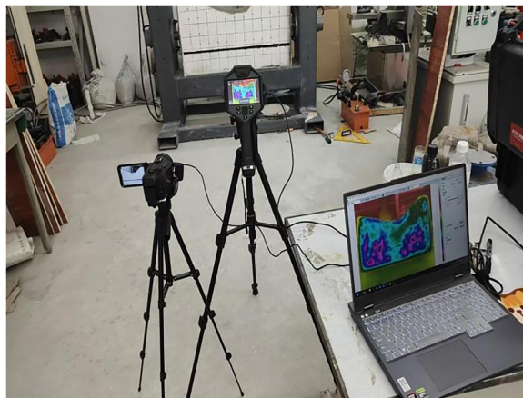
Figure 5. Surface damage monitoring
