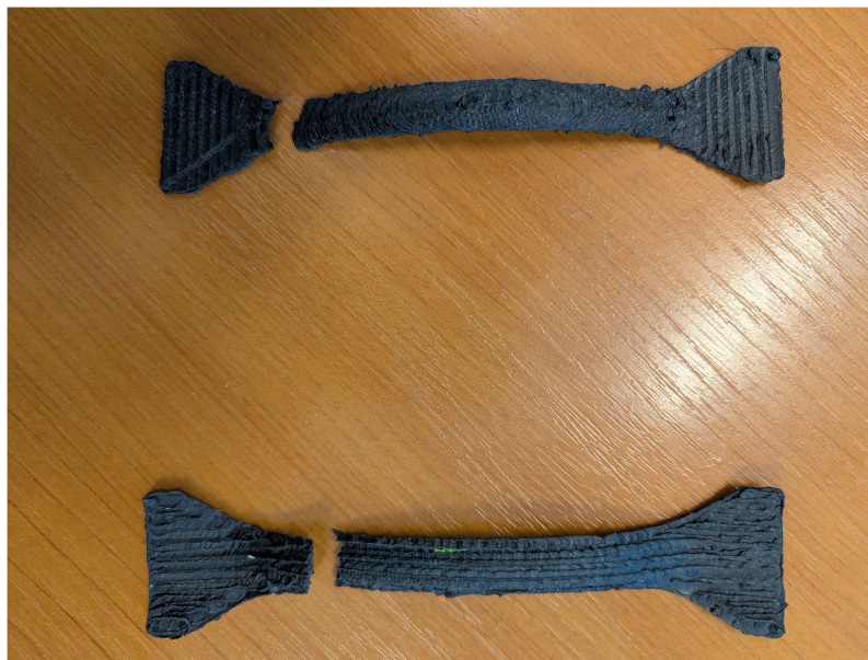
Figure 10. 3D printed samples: conventional/planar (upper image) and continuous/non-planar (lower image)
