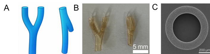
Figure 2. Morphological and structural characterization of DLP-printed GelMA vascular scaffolds. (A) CAD models of Y-shaped and curved vascular geometries used for printing. (B) Photographs of the corresponding printed GelMA scaffolds, showing good structural fidelity and continuous tubular morphology. (C) Cross-sectional SEM image of the printed tubular scaffold, revealing a well-defined circular lumen of approximately 1 mm in diameter and a layered wall microtexture characteristic of the DLP printing process
