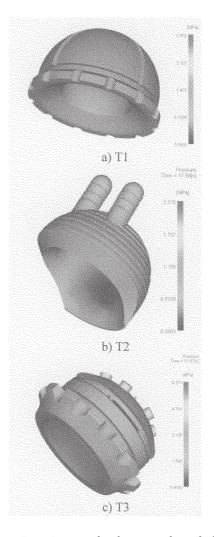
Fig. 4. Pressure distributions at the end of filling
