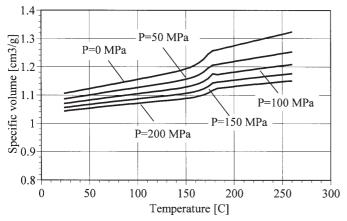
Fig. 1. Specific volume as a function of temperature
