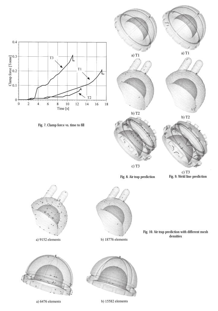
From figures 8 and 9, it has been observed that the number of the defects (air traps and weld lines) is smaller in cup T1 than those in cups T2 and T3, respectively.
