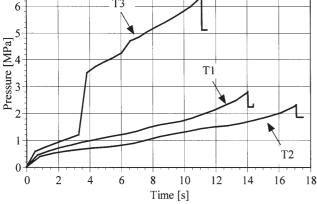
Fig. 5. Pressure vs. time to fill the acetabular cups at the entrance of the cup
