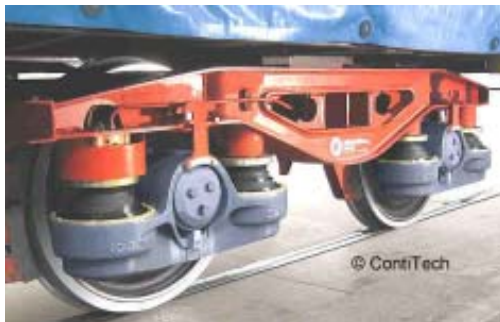
Fig. 4. Y25 freight bogie with rubber suspension [7]
