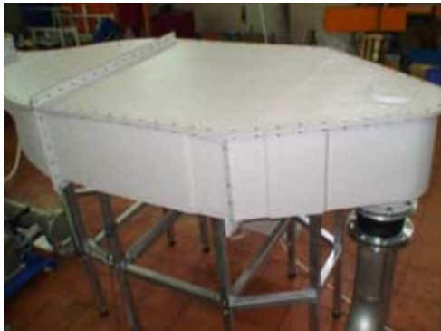
Fig. 4. Water tunnel sections made of FRP
