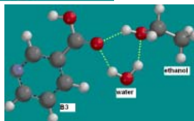
Fig. 8. Possible intermolecular hydrogen bonds formed between B 3 -water-ethanol (red -oxygen atoms, gray-carbon atoms, white-hydrogen atoms, blue-nitrogen atom, broken yellow line- hydrogen bonds)
