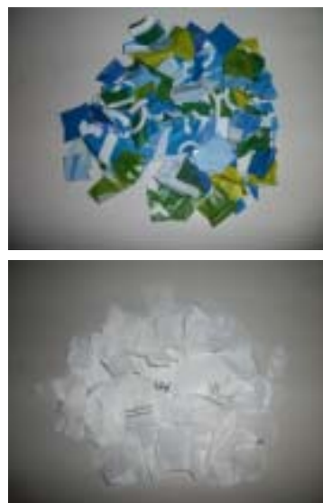
Fig. 2. Painted bag after having been cut into pieces (a); Non painted bag after having been cut into pieces (b)
