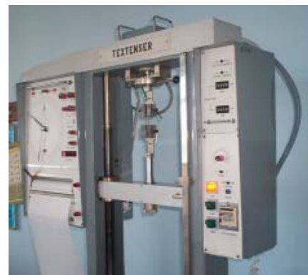
Fig. 7. The Textenser device used for tensile tests
