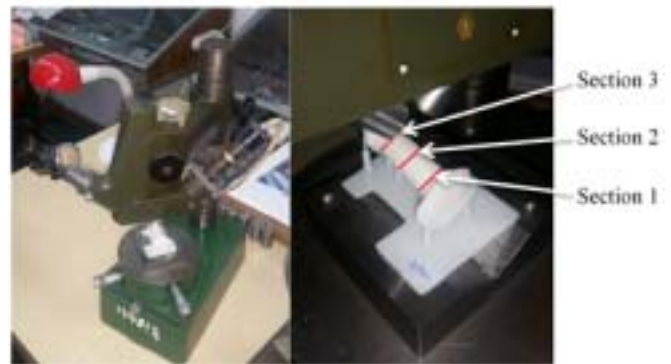
Fig. 6 Surface roughness measurement of custom spinal implant concept 1
