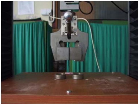
Fig.2. The three-point bending tests on Zwick/Roell testing machine
