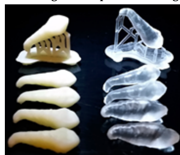
Fig. 2. Group A resin replicas (left) and group B resin replicas (right), with and without supporting structure
